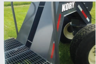
Extra heavy duty gooseneck with protected open hose inspection area.
