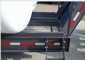
Elevated slip resistant platform with handrails allows easy access to both valves.
